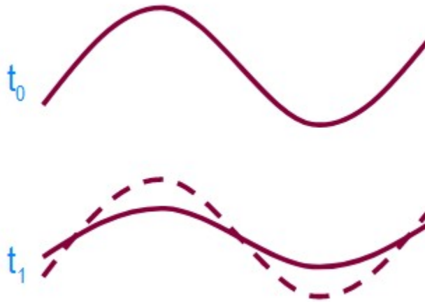
Figure 13: Single-sediment diffusion and schematic evolution of topography.
